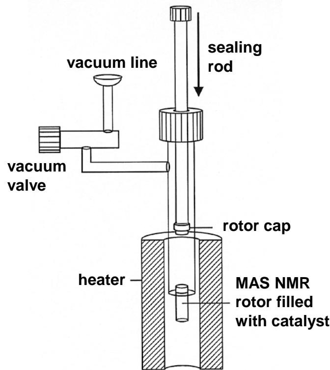
dehydration and loading of the catalyst inside the glass insert (e.g. commercial Wilmad MAS NMR inserts for 4 mm and 7 mm rotors)
