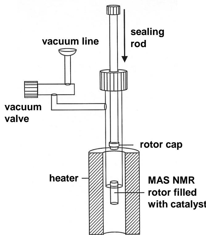
dehydration and loading of the catalyst inside the glass insert (e.g. commercial Wilmad MAS NMR inserts for 4 mm and 7 mm rotors)
