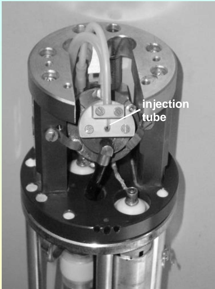
Bruker 7 mm MAS NMR probe modified for experiments under flow conditions (left) and special tools for shaping the catalyst to a hollow cylinder (bottom)
