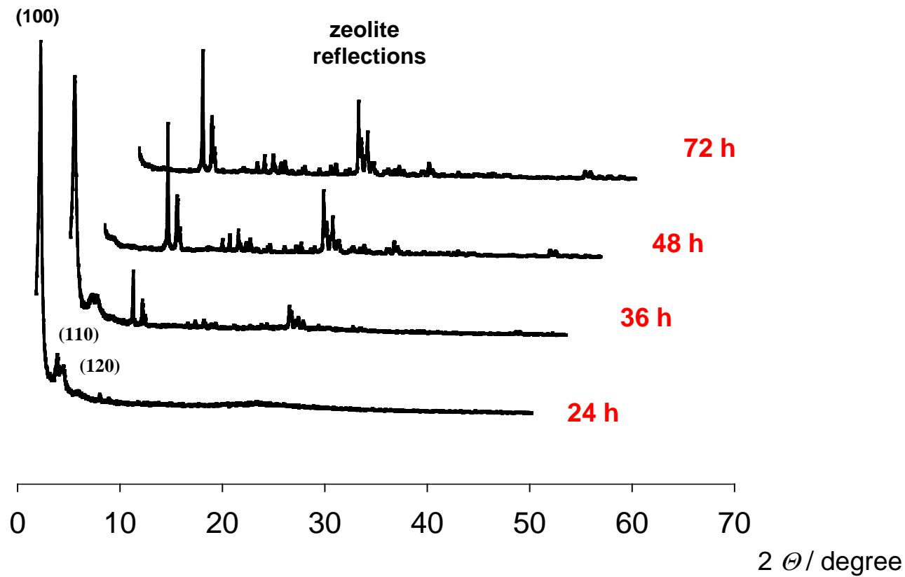
→ increasing zeolite domains with increasing conversion time
