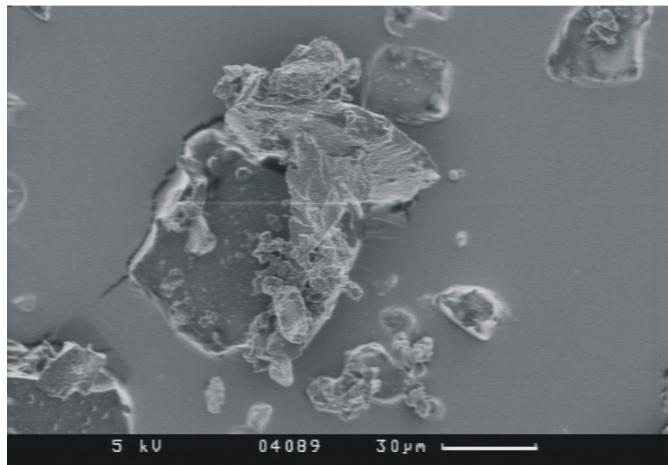
zeolite particles (< 0.5 µm)
