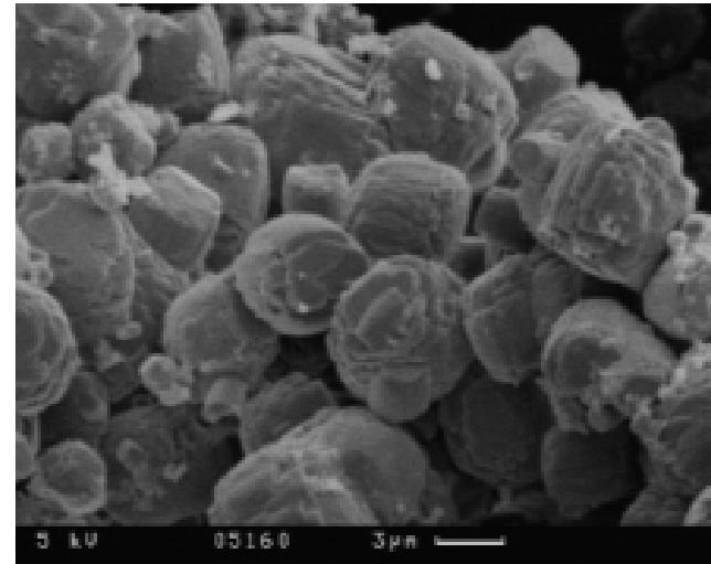
→ **meso-structured material is totally converted to ZSM-5 crystals**
