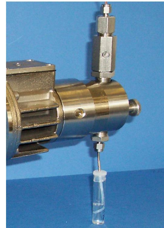
pump Mikro g/5 of Fa. ProMinent, Germany, for single pulses with volumes of 2 to 50  $\mu\text{l}$
