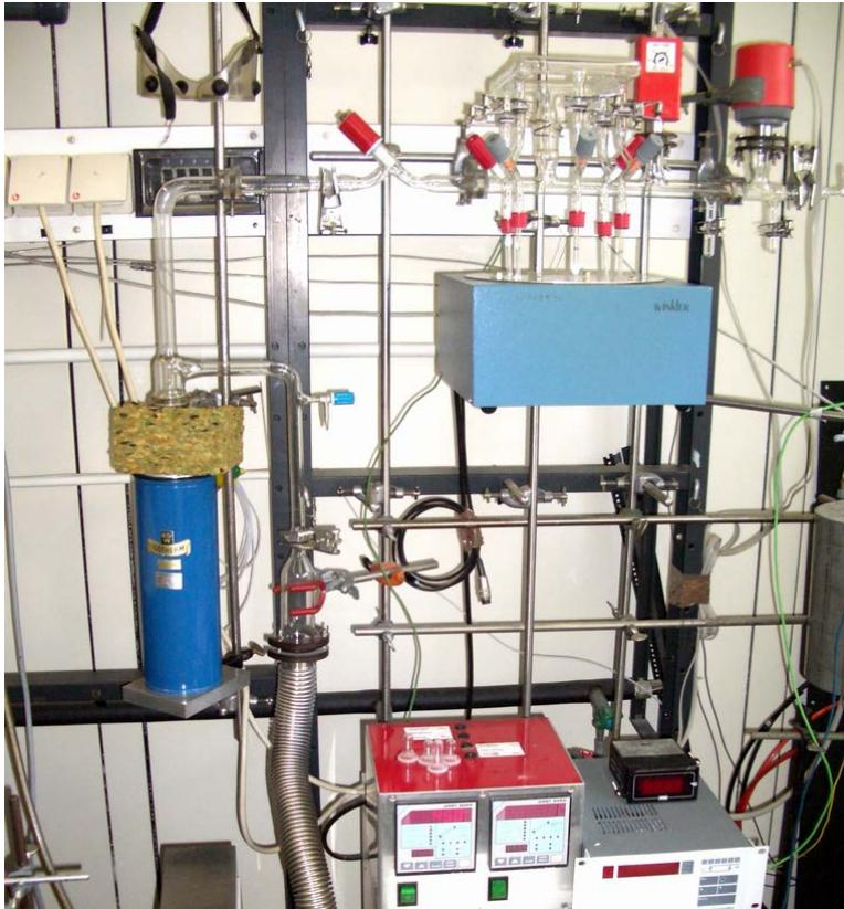
vacuum line for dehydration of catalyst samples in glass tubes at elevated temperatures (often 673 K)
