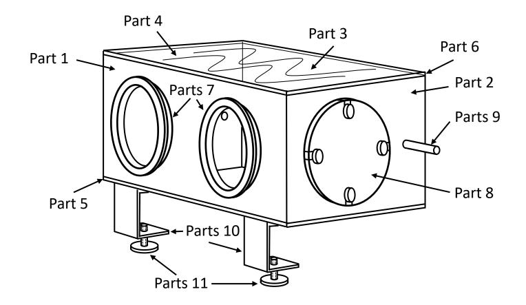
Part 1: material plexiglass, polyvinyl chloride (PVC) or aluminum
