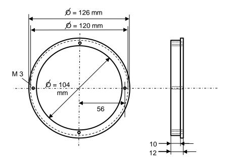
Part 8: material polyvinyl chloride (PVC) or aluminum
