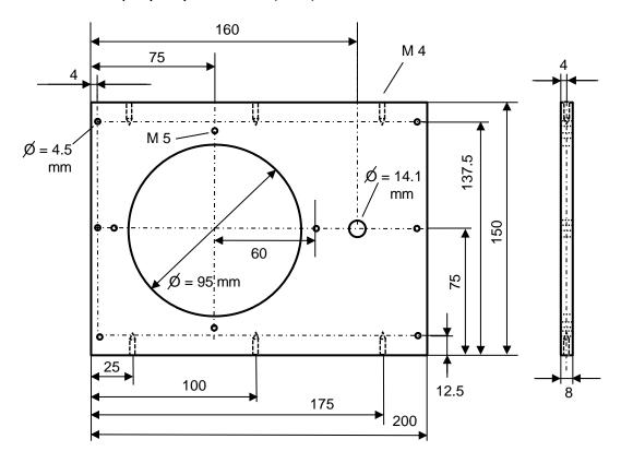
Part 3: material polyvinyl chloride (PVC) or aluminum
