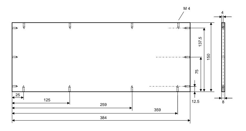
Part 4: material polyvinyl chloride (PVC) or aluminum
