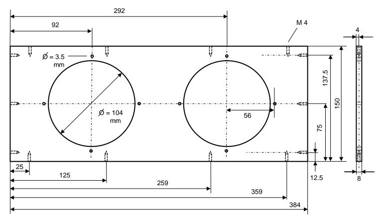
Part 2: material polyvinyl chloride (PVC) or aluminum
