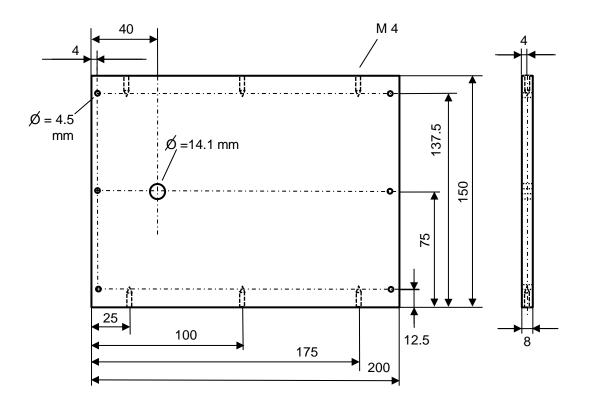
Part 5: material polyvinyl chloride (PVC) or aluminum
