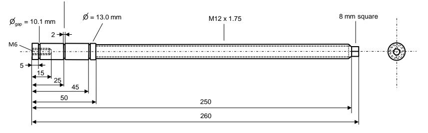
annular gap for VITON O-ring 10 mm x 2 mm (OD 14 mm)
